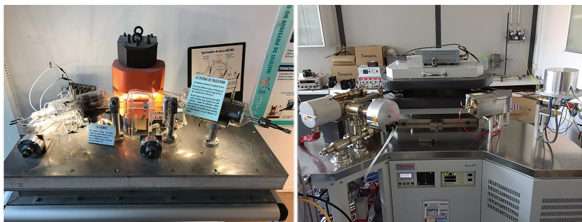
Figure 1.2 Left: Glass mass spectrometer of the type developed by John Reynolds. This instrument was bought by Claude Allègre and is now on display at the Institut de Physique du Globe de Paris. Photo credit: G. Avice. Right: A modern metal noble gas mass spectrometer at the CRPG (MC SFT by Thermo Fisher Co). Photo credit: B. Marty.
