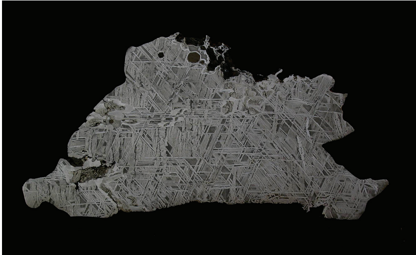
Figure 10.8 The Widmanstätten figure or pattern of this iron meteorite is due to the differential etching of kamacite ( \alpha -iron with about 5.5 % nickel) and taenite ( \gamma -iron with between 13 % and 48 % nickel). The kamacite is in the form of plates that have exsolved, parallel to the faces of the octahedron, from taenite. The width of the kamacite lamellae is a measure of cooling rate (photo credit: A. Pack).
